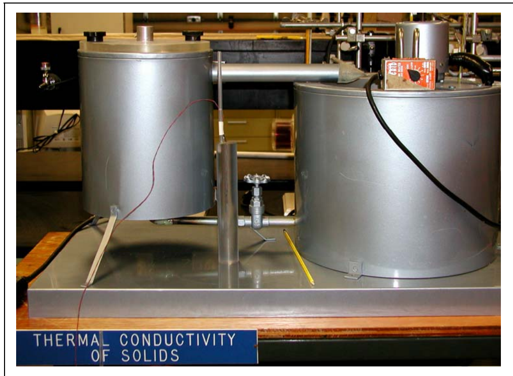
Figure 1. Thermal conductivity apparatus, with sample chamber (left), hot water bath, immer-
