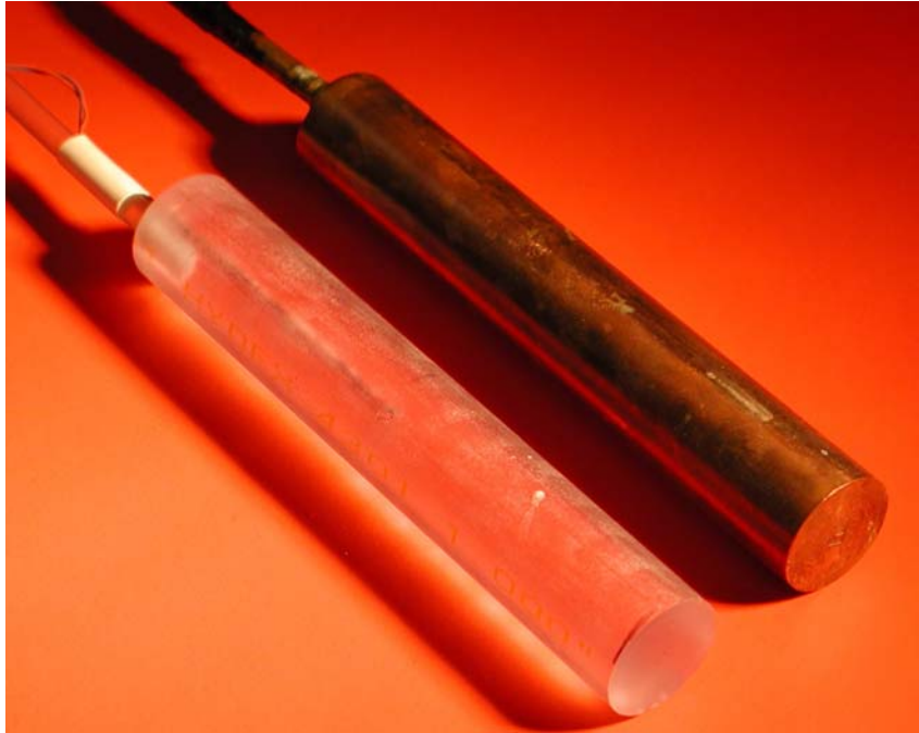
Figure 2. Polycarbonate and phosphor bronze (cylinder “F”) test specimens.
