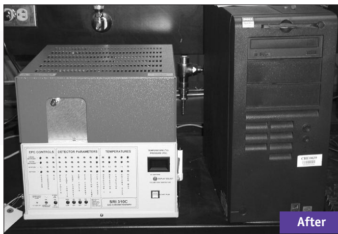
New SRI 310C gas chromatograph provided through ChE Academy support
