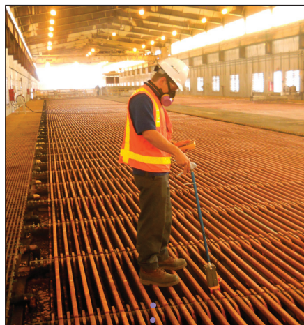
Jaron Meyer ..... pictured in a tankhouse where stainless steel cathodes are plated with 99.999% copper, worked for Freeport McMoran Copper and Gold on the hydro-metallurgical processing side of the mine in Morenci, Arizona.
