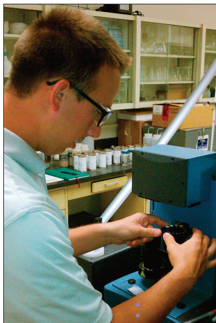
Glenn Hafenstine ..... worked for Burns & McDonnell in Kansas City, testing gypsum slurries from scrubbers at power plants.
